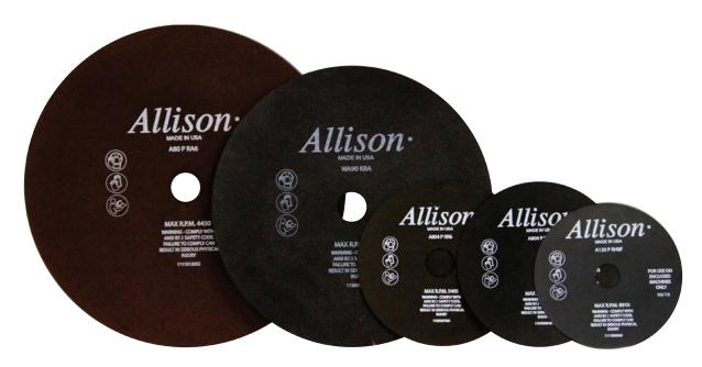
The cutting of electrical contact disc from tungsten rod is commonly done wet with rubber bonded wheels 6 or 7 inches in diameter and from .013 to .017 inches thick, held to thickness tolerance of plus or minus one-thousandth of an inch. Similar wheels are used for accurate cutting of very small rod and tube sections and for cutting thin slots in various materials.
