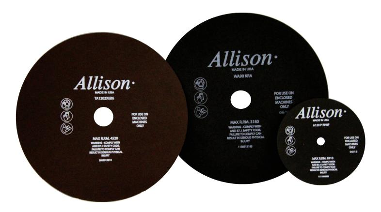
Rubber bond, fine abrasive particles, and filler materials selected to maintain a square or slightly concave cutting face make Allison abrasive cutting wheels ideal for cutting thin-wall metal tubing with bsolute minimum burr. Most Allison rubber bonded heels can be used with or without coolant. Cutting with coolant provides the best cut quality, and greatest number of cuts per wheel. However, cutting with coolant provides the best quality and greatest number of cuts per wheel.
